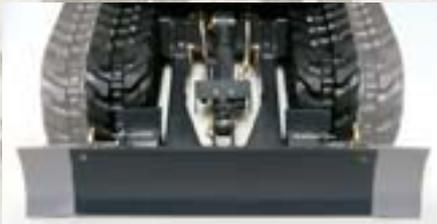
With the simple removal of one pin, its quick-fold blade adjusts in size instantly.
